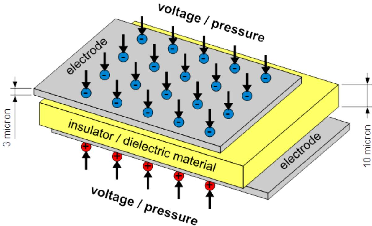
*Pumping electric charges with voltage really results in a mechanical pressure on the insulator layer. Applying too much voltage will cause it to break down (electrically, not from the mechanical pressure itself).*
