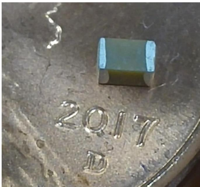
**Figure 1. EESstor .0805 MLCC displayed on a Penny**
