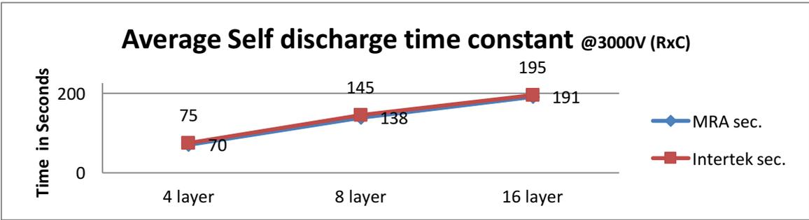
EEStor calculates that using the stacking methodology to keep resistance high, a stack of 320 layers would have a capacitance 140ηF and a time constant of 64 minutes giving the device a discharge duration of over 5 hours.
